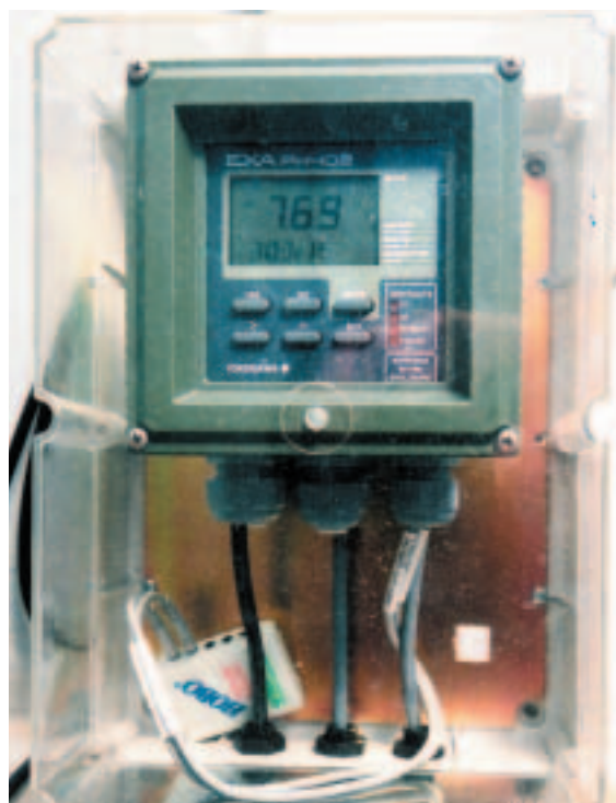
pH meter: An example of an automated pH meter linked to a system which treats the water to maintain a predetermined pH
